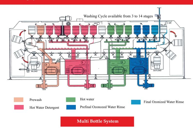
SEPPA has developed the most futuristic multi bottle system keeping in perspective of the variations in large bottle heights due to multiple sizes of large bottle varying from 3-6 gallon. SEPPA has developed the EVATS-1000-MBAA™ series (Multi Bottle Auto Adjustment™ System). In this series of SEPPA large bottling machine, multiple sizes bottles can be fed into the auto loader, washer, filler and capper. The auto loader is designed to load different sizes of bottles into the washing zone.
