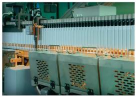
Different necks sizes of performs can be handled by a quickchange over of the preform holder and mantel.
